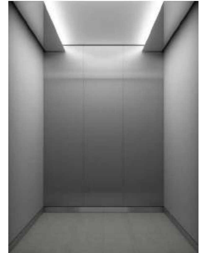
Ceiling ..... DL5 Panel: Mirror stainless-steel Lighting color: Cool white Walls ..... Rear: Hairline stainless-steel Side: Painted steel sheet [Y136D: Ash gray] Kickplate ..... Hairline stainless-steel Flooring ..... PR803: Gray
